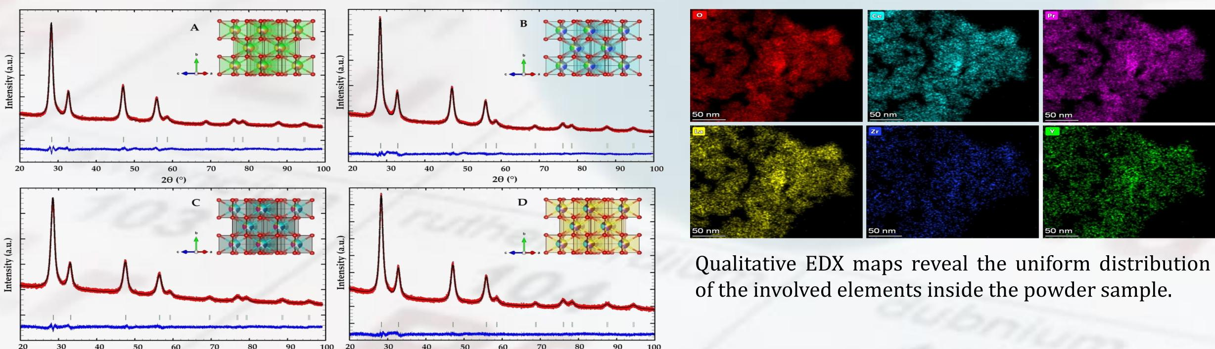
Rietveld plot of the investigated compounds: (A) CZLEY; (B) CZLPY; (C) CZEYG; (D) CZLPG. Along with Bragg reflections, the observed (red), calculated (black), and difference (blue) plots are shown for the fit of the PXRD pattern. In the insets of each figure, the fluoritetype crystal structure of the corresponding HEO is visualized.
