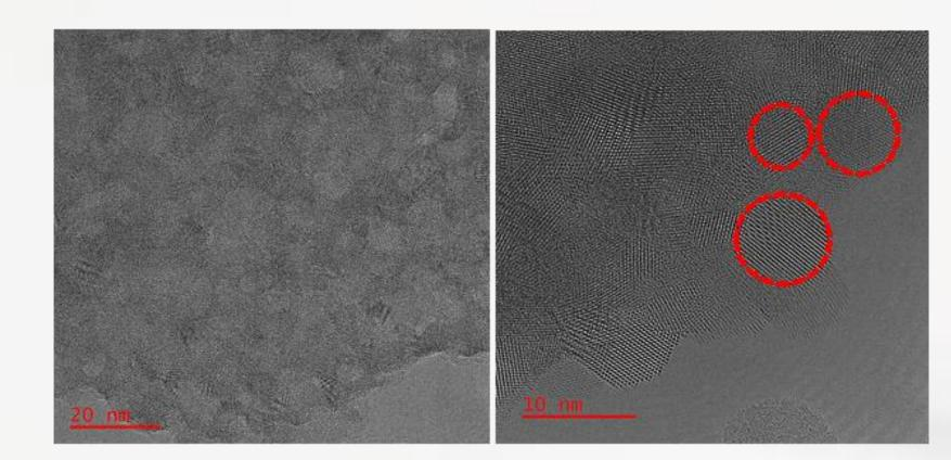
TEM/HRTEM images of CZLPY powder the sample at different magnifications confirms that average crystallite size is less than 10 nm
