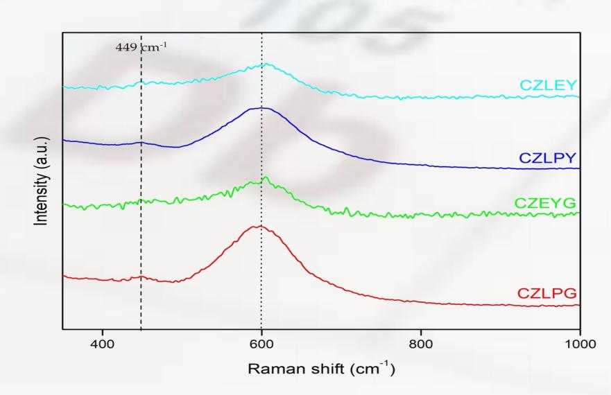
Raman spectra of the synthesized HEOs.  $F_{2q}$  band shift of ~15 cm<sup>-1</sup> is related to the expansion of the crystal lattice, the bond lenghts, and the formation of oxygen defects. Additional bands at  $\sim 600 \text{ cm}^{-1}$  are related to oxygen defects.
